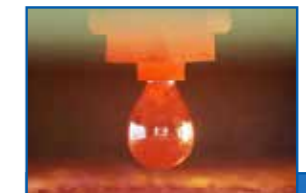
Molten aluminium droplet in NHD 700/TEC 700
