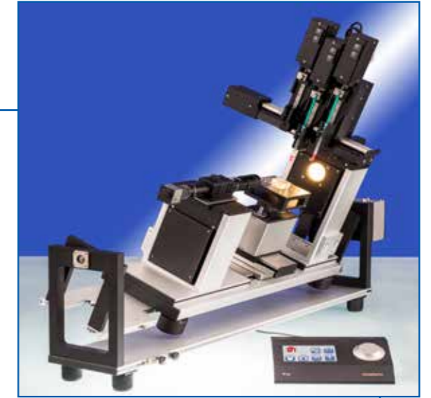
OCA 50Pro on tilting base unit TBU 95 with electronic multiple direct dosing unit DDE/3
