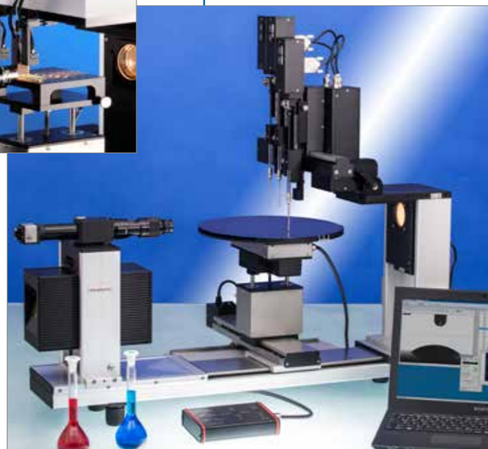
Fully automatic mapping on 12" wafer with OCA 35XLH, ETT/VAC, WTP 12/VAC and TD-DE/3
