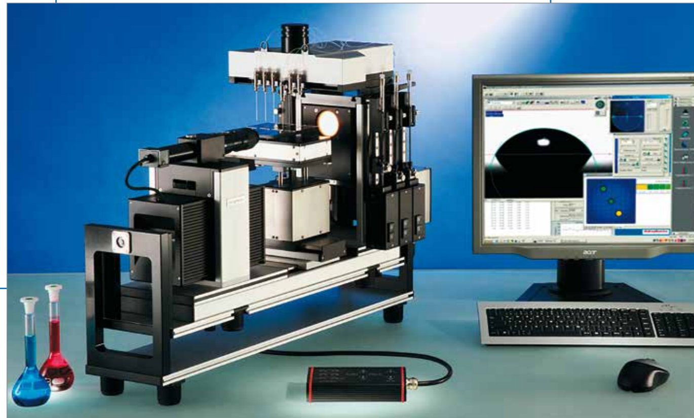
OCA 35/6 on tilting base unit TBU 90E with electronic turn table with vacuum fixation ETT/VAC and electronic multiple dosing system E-MD/6
