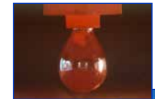
Molten aluminium droplet in NHD 700/TEC 700
